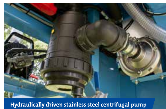
Hydraulically driven stainless steel centrifugal pump
